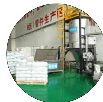
Raw materials dry and dehumidify to ensure the quality
