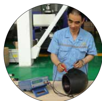
Strict resistance test of each electrofusion fitting
